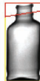
Figure 7: Detection of missing cap
