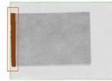
Figure 18: Wound dressing trapped within the seal
