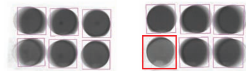
Figure 16: Twin lane inspection of six-pack yoghurts with one low fill
