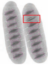
Figure 4: Shows two garlic baguettes with one low-fill
